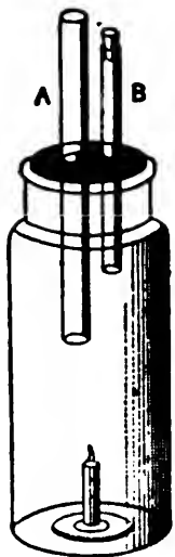
FIG. 145.— Showing the neces- sity of two currents to sustain combustion. (Munson.)
